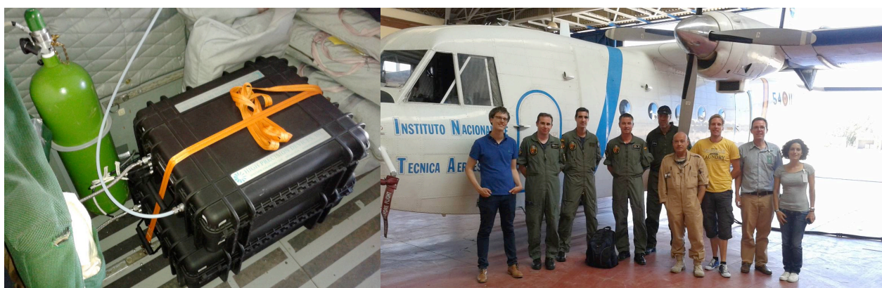
Figure 2. Left picture: quasi automatic air sampler installed on board the INTA's aircraft. Right picture: group picture (crew and some of the technicians and scientists involved in this campaign) and aircraft.
