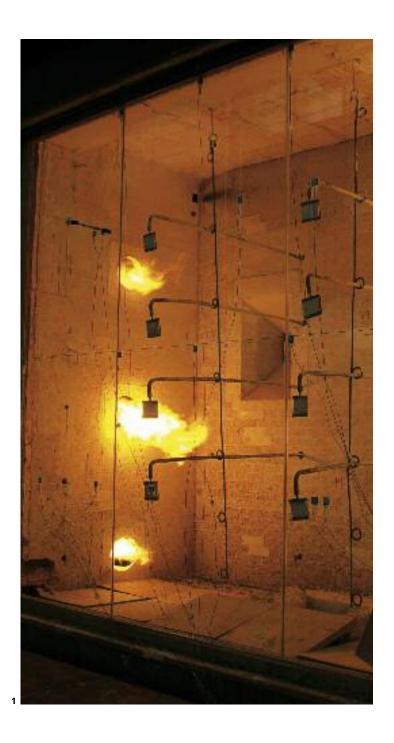
Empa has been burning for 40 years. In the Fire Technology Laboratory at Dübendorf, the most varied components are turned into ashes. This is done not just to gain knowledge about how materials and components behave when burning, but also to optimise them. In future, even computer models should help predict the materials' behaviour in the event of fire.
