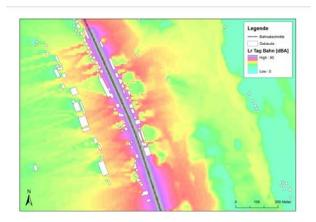
Noise levels along the track due to rail traffic can be predicted accurately using the computer model. (Source: LCC Consulting)
