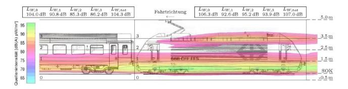
Noise is generated at several different locations along a train composition: primarily at the wheels, but also higher up at the exhausts of the engine cooling system on the roof. (Source: Sulzer Innotec)
